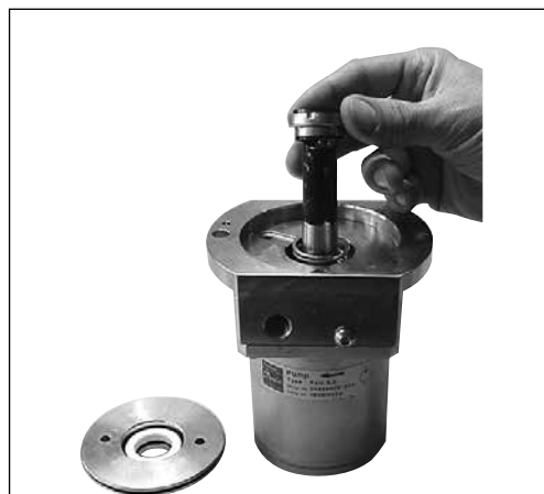
23. Wet the shaft seal and slide it over the bush.
