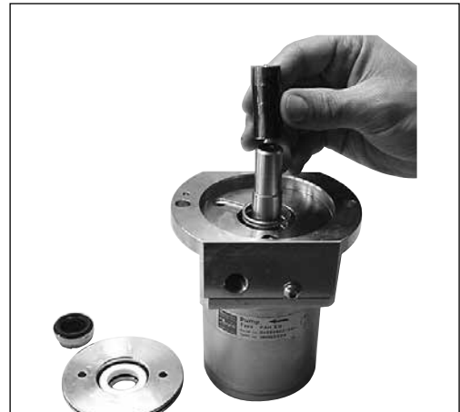
22. Fit the hollow bush onto the shaft.
