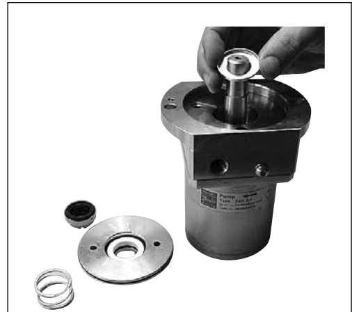
20. Mount the washer with the edge pointing upwards.
